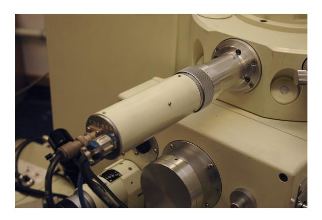
The perspex light pipe can drop out of position when fitting, reducing the light collected. Fit the light pipe loosely in the adaptor using plastic centring disk. Engage the other end into the optical window recess in the electron microprobe and push the adaptor forward so it can be mounted.
