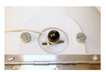
5. Turn power on at the wall and turn on machine. The mill must be on before pouring material into the hopper.
